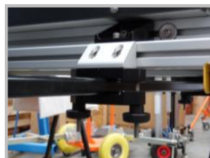
Aluminium frame and brackets for roof bars
