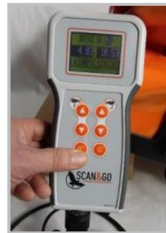
Simply press a button, the system proceeds automatically reaching the horizontal position on both axes.
